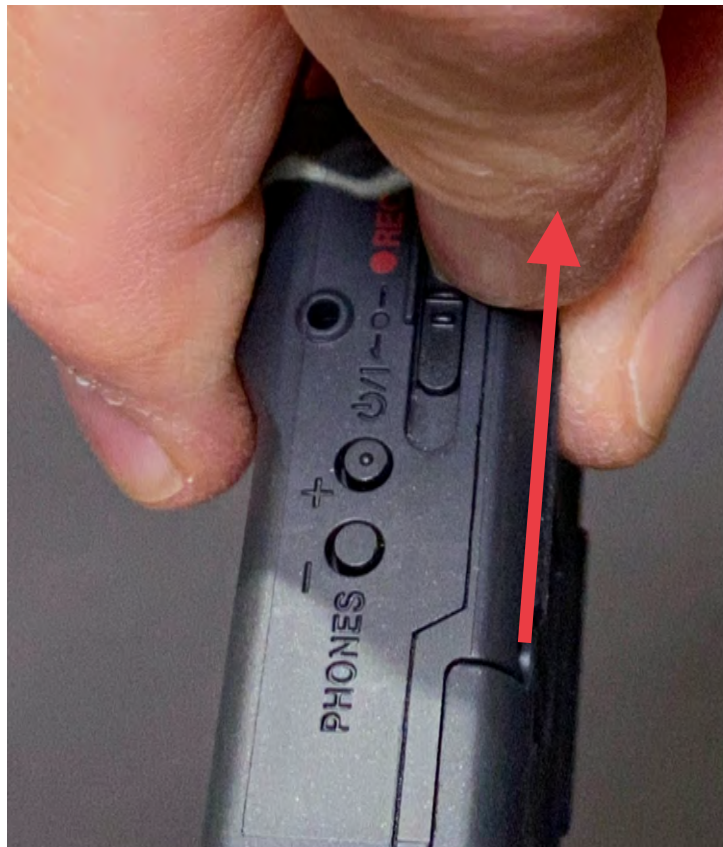
3. START RECORDING: Use your fingernail to pull UP the slider and hold for 3 seconds until the display shows a CIRCLE.
